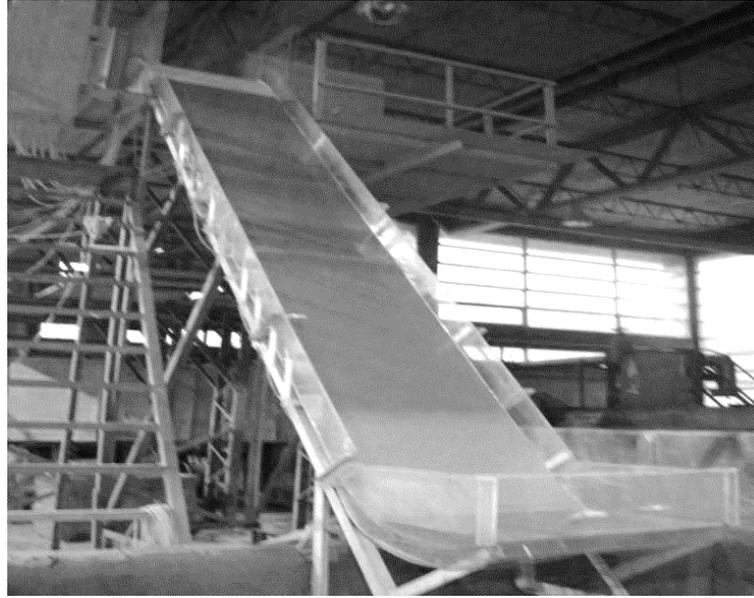
**Figure 1.** Hydraulic Model of Laleli Dam and HEPP [20]
